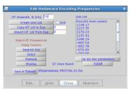
Uncheck lock to edit the line list. Place the cursor on the peak to be added or removed and click <u>Select</u> or <u>Remove</u> as appropriate. Click <u>Set list into parameters</u> save the Hadamard frequency list in the Data directory using <u>Save in Datader</u>, and close the dialog box. This frequency list will be used for all subsequent Hadamard experiments with PROTON indirect dimension.
